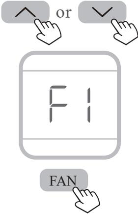
Press the or button to switch parameter code to “F1”. And short press the button to enter the unit address setting interface.
