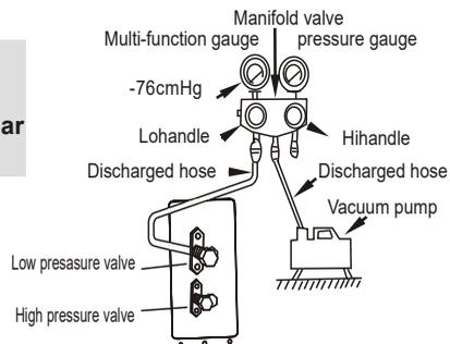
1. Connect the hose of manifold pressure gauge to the maintenance port on the low pressure valve of outdoor unit.
