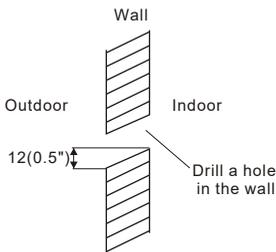
**NOTE:** When drilling the wall hole, make sure to avoid wires, plumbing, and other sensitive components. The drainpipe outlet should be at least 50mm (1.9") above the ground. If it touches the ground, the unit may become blocked and malfunction.
