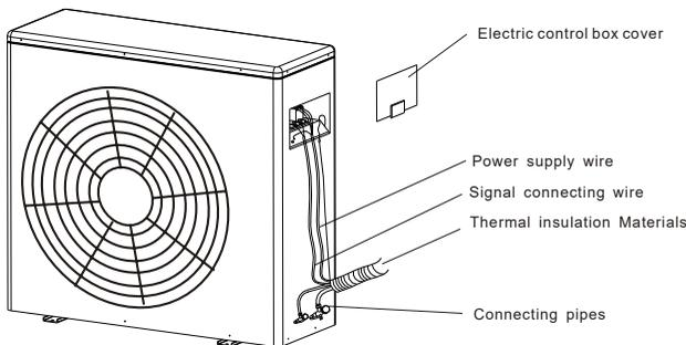
2. Connect the power connection cord to the terminal board. Wiring should fit that of indoor unit.
