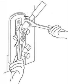
5. While firmly gripping the nut, use a torque wrench to tighten the flare nut according to the torque values.
