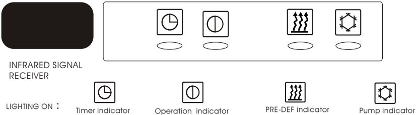
Timer indicator : ON when preset time for switching ON/OFF the unit
