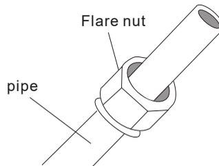
4. Remove PVC tape from ends of pipe when ready to perform flaring work.
