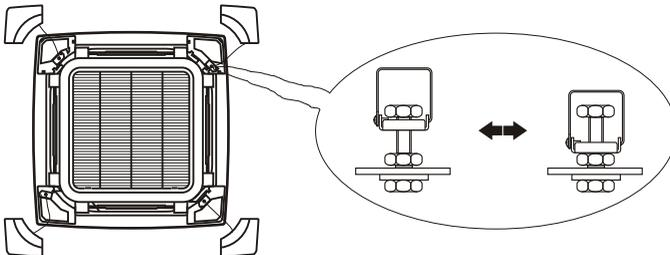
**NOTE:** Tighten the screws until the thickness of the sponge between the main body and the panel reduces to 4-6mm (0.2-0.3") The edge of the panel should be in contact with the ceiling well.
