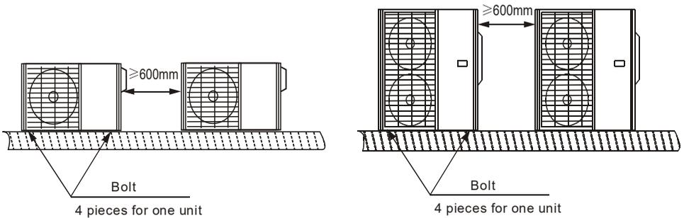
**NOTE:** The minimum distance between the outdoor unit and walls described in the installation guide does not apply to airtight rooms. Be sure to keep the unit unobstructed in at least two of the three directions (Front,Left,Right). (As shown on the right)
