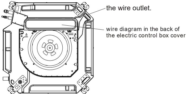
3. Connect the power connection cord to the terminal board. Wiring should fit that of Outdoor unit.
