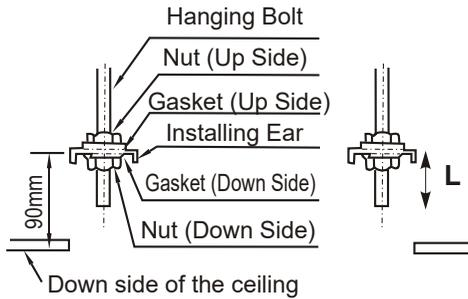
**NOTE:** Ensure that with the indoor unit is level. The unit is equipped with a built-in drain pump and float switch. If the unit is tilted against the direction of condensate flows (the drainpipe side is raised), the float switch may malfunction and cause water leakage.
